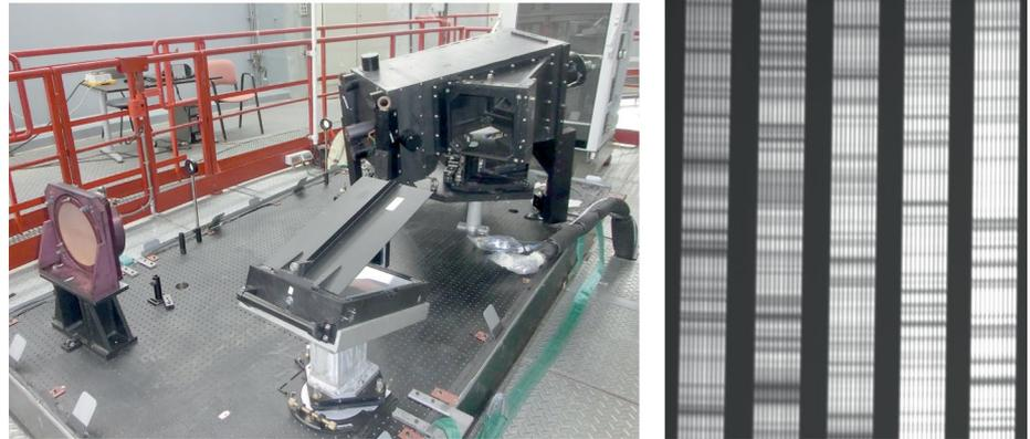
**Fig. 1** | A view of and through HORuS. Left: HORuS in the Nasmyth platform of GTC. Right: a spectrum of solar light scattered through the Earth's atmosphere. Credit: Félix Gracia Témich (left panel).
