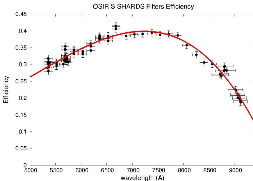
Fig. 2. SHARDS filters efficiencies measured during the development of SHARDS survey at the GTC (points). A polynomial fit to the data (red line) has been done to obtain a  $1\text{\AA}$  sampling. Error bars show both the efficiency uncertainties obtained from the standard star measurement and the filters' wavelength coverage (FWHM).
