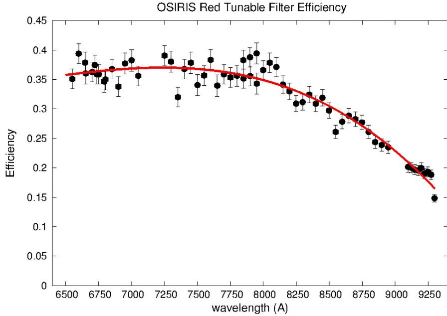
Fig. 1. RTF's efficiencies measured during OSIRIS commissioning (points). A polynomial fit to the data (red line) has been done to obtain a  $1\text{\AA}$  sampling. Error bars show the efficiency uncertainties derived from the standard star measurements.
