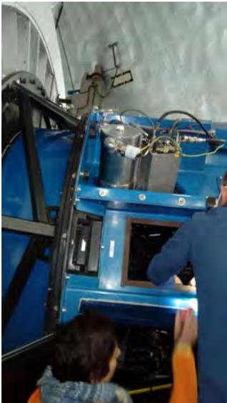
Fig. 12 Introducing NEFER scanning FP into OSIRIS wheels.
