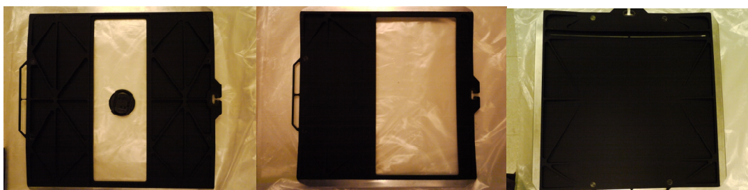
Figure 1.3.- From left to right, charge shuffling mask selecting the central 1/3 of the detector lines (the central black circular piece is shown just for reference), frame transfer mask selecting the half of the detector exposed, and the fast photometry mask with the decentered slit of 3 arcseconds width.
