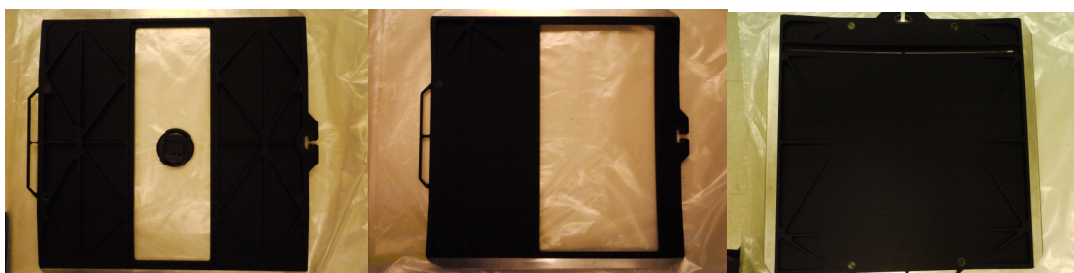
Figure 1.3.- From left to right, charge shuffling mask selecting the central 1/3 of the detector lines (the central black circular piece is shown just for reference), frame transfer mask selecting the half of the detector exposed, and the fast photometry mask with the decentred slit of 3 arcseconds width.
